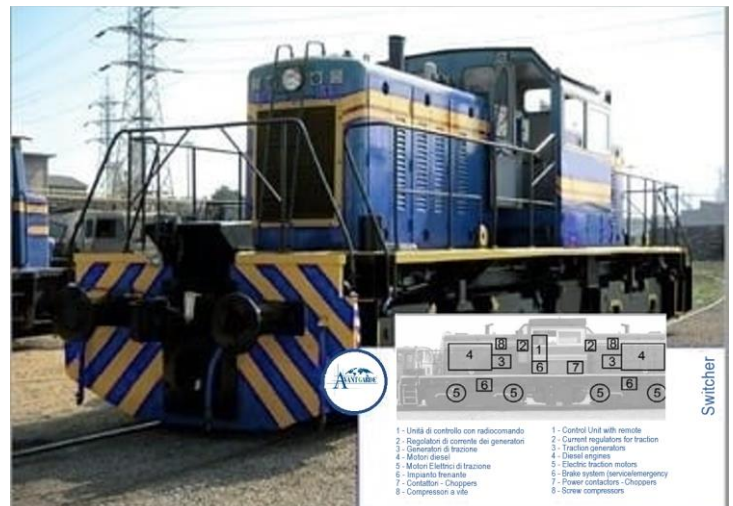
Switcher equipped with remote telemetry system TCAVi4.0
